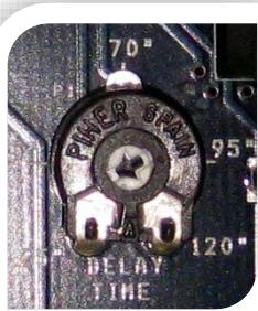
The **DELAY TIME** trimmer enables the user to set the duration (from 20" to 120") after which the acoustic and visual alarm signals are to be shut off (if the flashing light is installed) automatically.
