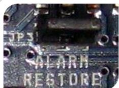
**ALARM RESTORE** Jumper (for automatic reset) active: the acoustic alarm and flashing light (mod. UNIT ALARM 2) are deactivated when the cause of the alarm is eliminated.
