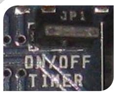
**ON/OFF TIMER** Jumper (to disable the alarm timer) not active: the siren and flashing light (mod. UNIT ALARM 2) continue to operate until the alarm condition is eliminated.
