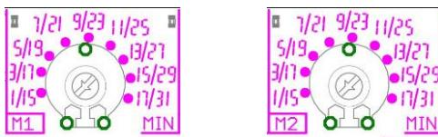
The “MIN” trimmer is used to adjust the minimum motor current for protection against the risk of dry run, for added protection or when minimum level floats or probes are not required.
