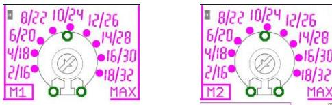
The "MAX" trimmer enables adjustment of the maximum motor current, over which the system protection trips due to current overload.
